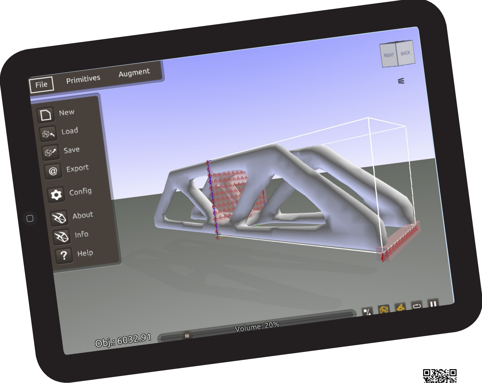
Screen shot from the TopOpt 3d App downloadable from the App Store.
