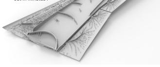
Aerial view of the optimized load carrying structure of a Boing 777 wing.
