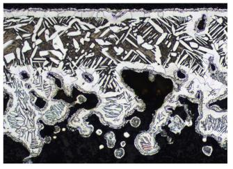
New methods for surface hardening titanium can solve the problem with wear resistance for the material and open up for a wide range of new applications. Left: A microscope image of a cross section of a pulley wheel before hardening. Right: The same cross section after the new hardening process, in this case the surface hardness has increased 5 times. Images from Emilie H. Valente's MSc project.
