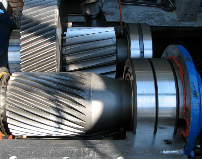
The photo shows the placement of the bearings and gears inside the nacelle of the wind turbine. Photo: Mogens Hvid
