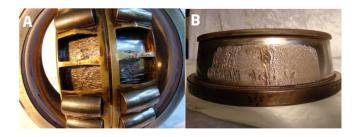
The photos show typical failure and damage of bearings which can be induced by so-called white etching. White etching cracks start below the surface and eventually leads to severe damage. The specific occurrence of the damage is difficult to predict, and the cracks may cause a complete breakdown of the wind turbine.
