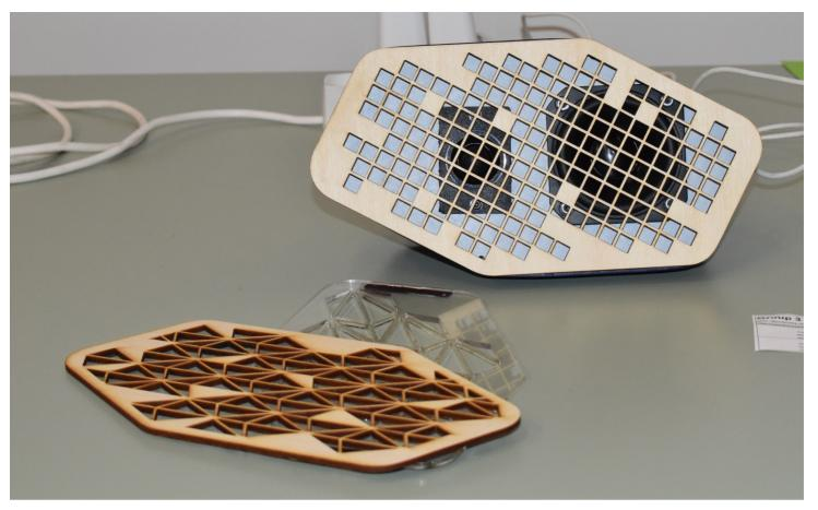
A wireless, 3D printed loudspeaker made by a student team at the BSc course "Mechatronics Engineering Design". Bang & Olufsen supplied the hardware for the prototypes.
